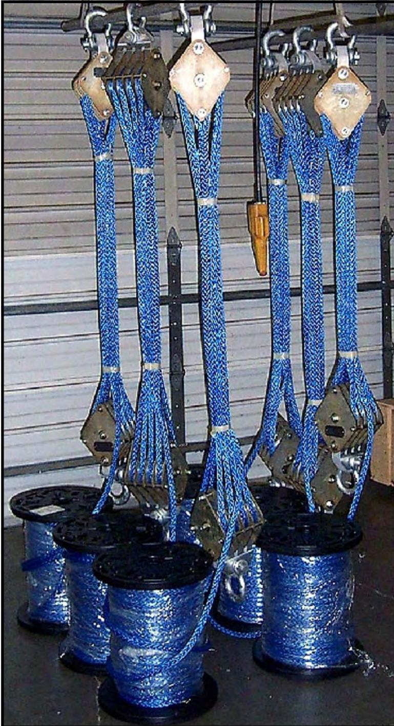
8 Part block and tackle ready for use. This set of block and tackle has been specifically designed for the line stringing industry with a robust, simple design.
